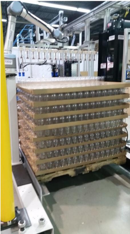
The system can be moved into position, set up, and quickly put in production. The Half-Cube palletizer provides maximum flexibility and efficiency and can be configured to pack all necks up or all
